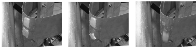
Fig. 11 Snap shots of the de-icing (at 10°F) sequence after triggering the proposed method in 30, 80, and 127 s.
